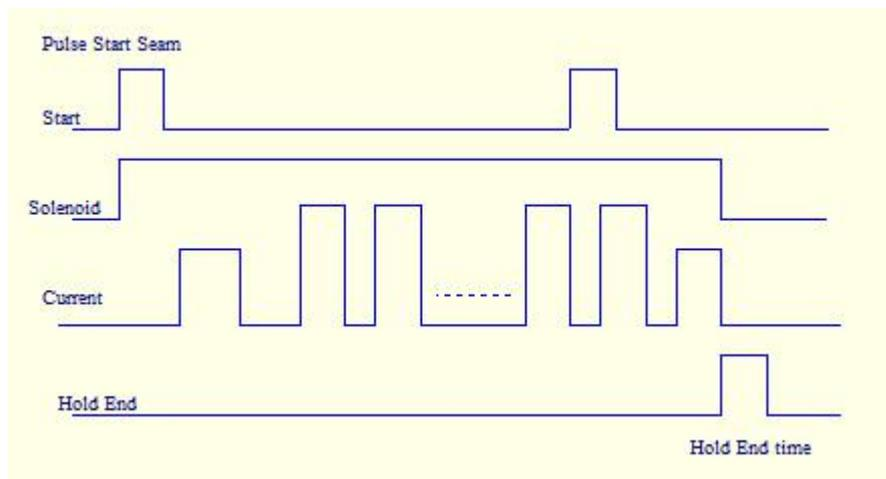
When the welding controller is in seam welding mode, the welding current switches between up to 4 “segments”, which represent 4 different currents and timing pairs. When the “SEAM TIMING” parameter is ON, the Cycle Current switch is valid, and is used to cycle between the segments in the order SEAM 1, 2, 3, 4.
