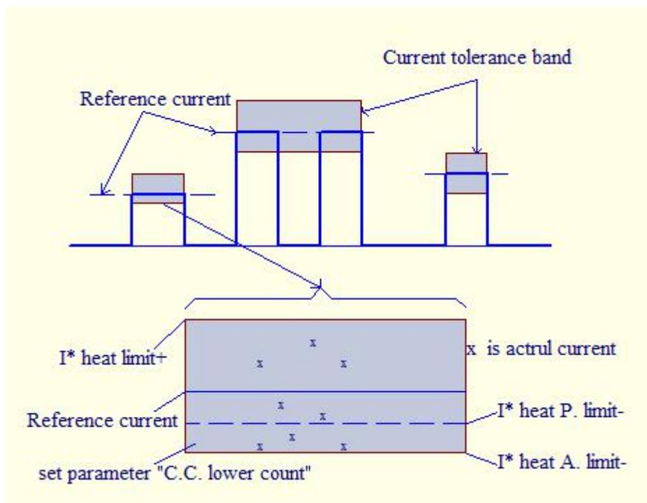
1.  **$I^*$ HEAT REFERENCE** (\* =1, 2 or 3, corresponding to preheating, welding and reheating respectively) : For each of the three weld steps, this is the reference current that is the baseline for comparing actual currents in order to determine if the weld current is satisfactory.
