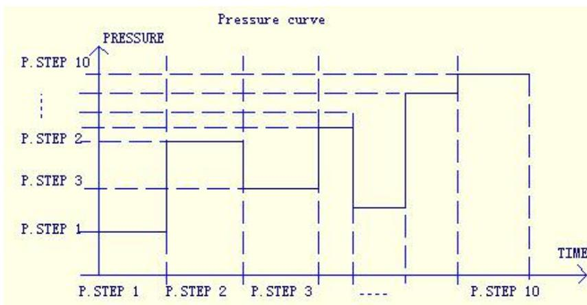
2. Pressure of Pressure Section 1: Pressure section 1 is relative to the maximum pressure percentage, in the same logic, every pressure section corresponds to one pressure value. It uses the “pressure-based value” as the standard scale for the maximum output pressure value.
