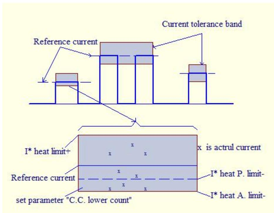
1. **I \*HEAT REFERENCE** (\* =1, 2 or 3, corresponding to preheating, welding and reheating respectively)
