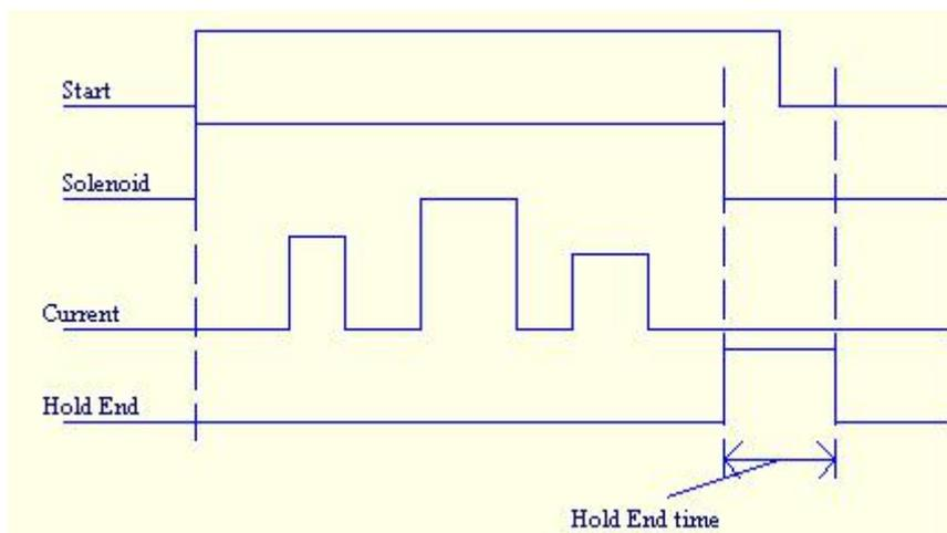
2. **Repeated Spot Welding:** during the process of repeated spot welding, the welding proceeds according to programmed parameters as long as the Start signal is asserted. In each weld cycle, the solenoid actuates, the weld is performed and the solenoid valve is released. At this time a delay equal to the OFF time begins. After the OFF time has elapsed, the solenoid valve will close, and resume the next welding process. The following figure shows the process for Repeated Spot Welding:
